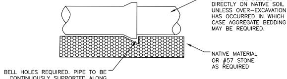
CONTINUOUSLY SUPPORTED ALONG LENGTH OF BARREL EXCEPT AT BELL
