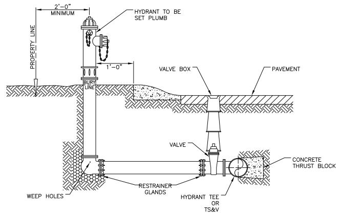
PLACE GRAVEL TO 6" ABOVE WEEP HOLES, 18" BELOW WEEP HOLES AND 18" TOWARDS THE MAIN. ALSO 16" LATERALLY ON EACH SIDE.
